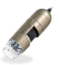
The AM4113TL-FVW is an ideal solution for inspection and working on objects of art where the usage of UV light is required. The long working distance of up to 15 cm enables the user to work under the microscope. This model offers a magnification of up to 90 times and switchable LED lights. The lights can be switched from UV to white light. The UV light supplies an excitation of 390~400 nm. It is equipped with a filter which blocks the returning UV light, resulting in images with natural colors.
