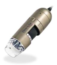
The AM4113T-FVW is suitable for inspection of paintings, ancient relics or other objects of art where UV light is required. It offers a high magnification (up to 200 times) and switchable LED lights – they can be switched from UV to white light. The UV light supplies an excitation of ~400 nm. It has a filter which blocks the returning UV light, resulting in images with natural colors.
